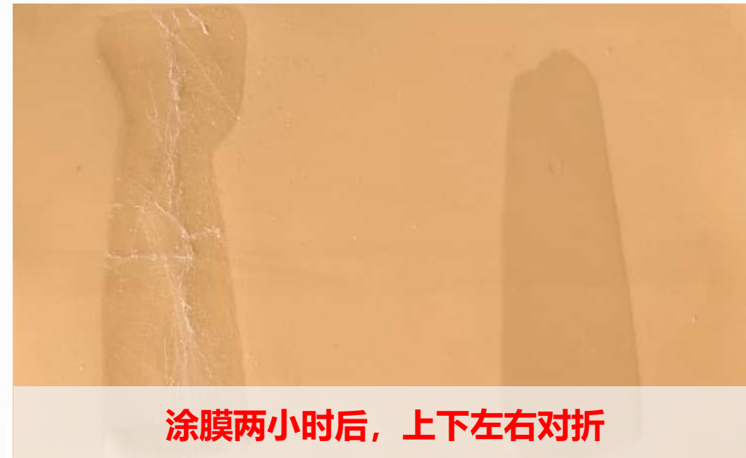
Fold the coating vertically and horizontally after 2 h
